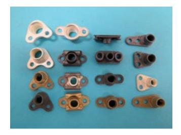
These are the most common mini rivet pattern nut plates made today which are elliptical at the end of the threads in order to make them "locking". They come in both steel and stainless steel types. Some are CAD plated, while others are lubricated. The high temp stainless steel ones are silver plated or lubricated.
